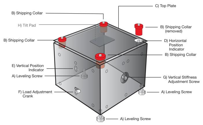
DO NOT REMOVE SHIPPING COLLARS UNTIL INSTRUCTIONS INDICATE. SHIPPING COLLARS MUST BE USED WHEN MOVING ISOLATOR.
