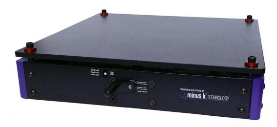
The tabletop, negative-stiffness CT-10 passive vibration isolator measures just over  $12.5 \times 2.7$  in. It delivers 0.5 Hz vertical and  $\sim 1.5$  Hz horizontal natural frequencies. Negative-stiffness isolators employ a completely mechanical concept in low-frequency vibration isolation and do not require electricity or compressed air. Applications include microscopy, microhardness testing, and laser/optical systems.
