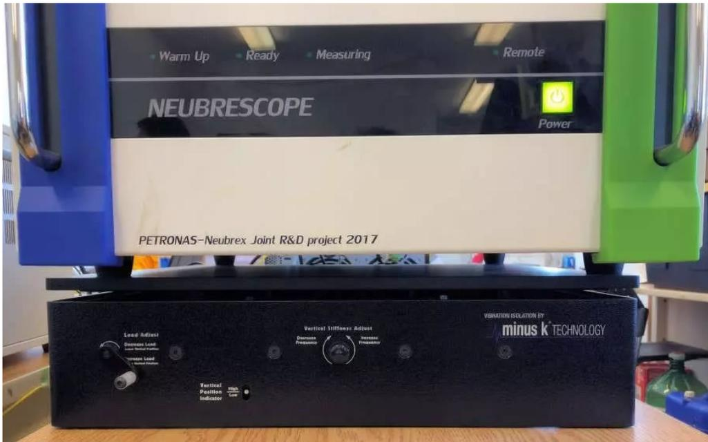
*Negative-stiffness vibration isolator beneath the Neubrescope.*
