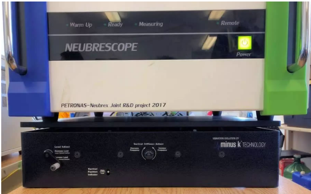
Negative-stiffness vibration isolator beneath the Neubrescope.
