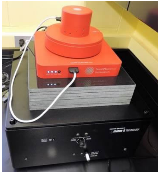
ezAFM+ supported by Negative-Stiffness vibration isolation.
